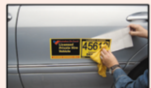
Slowly pull down the backing sheet and smooth down starting from hinged point.
